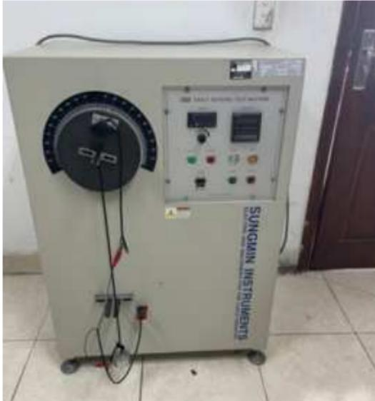
➤ Cable Bending Test Machine
